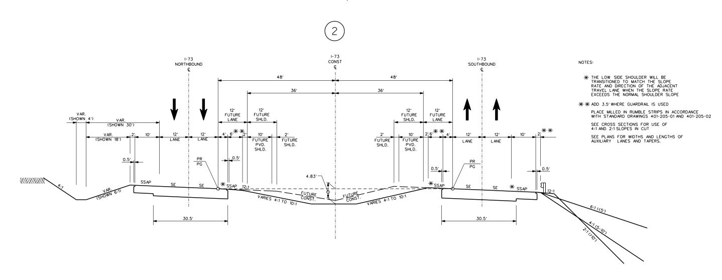
USE THIS SECTION ON 1-73 MAINLINE IN SUPERELEVATED SECTIONS
