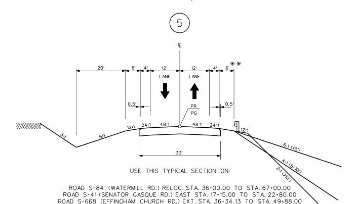
PG 33' USE THIS TYPICAL SECTION ON: DERRICK RD. RELOC. STA. 28+40.31 TO STA. 49+88.00 ROAD S-668 (EFFINGHAM CHURCH RD.) NORTH STA. 20+12.53 TO 28+50.00 ROAD S-668 (EFFINGHAM CHURCH RD.) SOUTH STA. 34+35.00 TO 36+10.08
