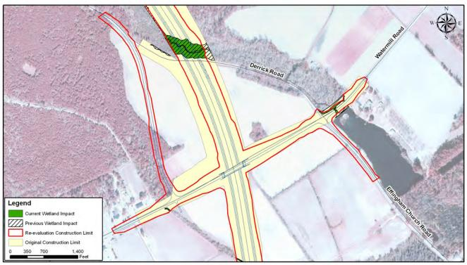
Figure 2-4: Derrick Road Re-alignment
