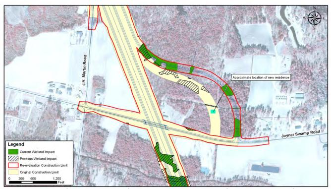
Figure 2-6: J.H. Martin Road at Joiner Swamp Road Frontage Road Re-alignment
