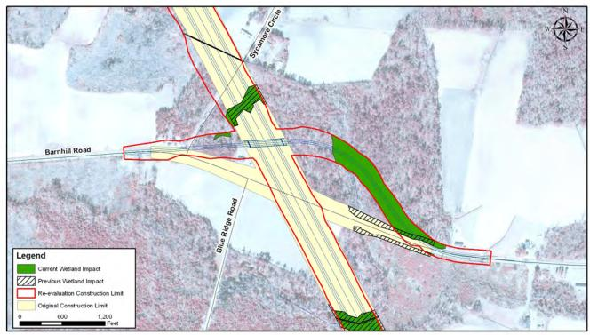
Figure 2-3: Barnhill Road Overpass Re-alignment
